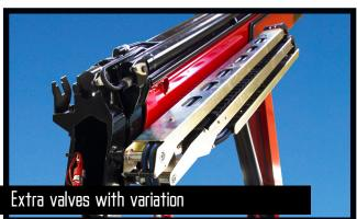
A well-known and usual hose routing to the end of the extensions means that 1 or 2 extra valves are fed in sturdy hose guides alongside the jib extension system. If further efficient protection of the hoses is required, 1 or 2 extra valves can be fed in internal hose reels and lie particularly well protected. In case of more than 6 hydraulic extensions or a reach of approx. 17 m, 1 or 2 extra valves will be fed in external, smooth-running and efficient hose reels.
