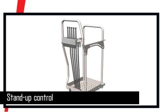
With stand-up control, the crane operator has an increased overview of the crane movements. Especially when loading and unloading the platform body with e.g. grab or pallet fork, the crane operator has the full view of both the platform body and the working area. The crane operator is protected by the HSL or HSL-E safety system which prevents the crane from hitting the operator on the stand-up platform
