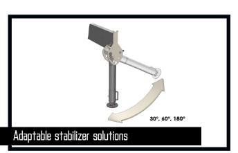
The stabilizer legs of the crane are to ensure stability - however they still have to be sturdy, easy to handle and must not take up too much space when not in use. Therefore you can choose between fixed stabilizer legs, manual swing-up stabilizer legs to 180° with gas spring or fully hydraulic swing-up stabilizer legs to 180°. Stabilizer beams can be freely selected as hydraulically extensible or manually extensible, also in connection with the sophisticated EVS stability monitoring.
