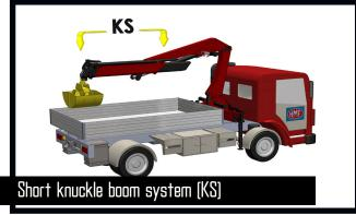
The short knuckle boom system (KS) is equipped with a shorter jib than a standard knuckle boom system. Thanks to a short knuckle boom system, the crane fitted with a grab can be stowed while extended in a platform body of 4 m without dismounting the grab. The lifting height close to the column is increased with more than 3 m and in this way offers the possibility of lifting tall items close to column. The boom system is available with 1, 2 or 3 hydraulic extensions.
