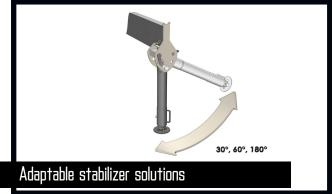
The stabilizer legs of the crane are to ensure stability - however they still have to be easy to handle and must not take up too much space when not in use. Therefore you can choose between fixed stabilizer legs, manual swing-up stabilizer legs to 30/60° or manual swing-up stabilizer legs to 180° with gas spring. Stabilizer beams can be freely selected as hydraulically extensible or manually extensible, also in connection with the sophisticated EVS stability monitoring.
