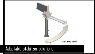
The stabilizer legs of the crane are to ensure stability - however they have to be easy to handle and must not take up too much space when not in use. Therefore you can choose between fixed stabilizer legs, manual swing-up stabilizer legs to 180° with gas spring or fully hydraulic swing-up stabilizer legs to 180°. Stabilizer beams can be freely selected as hydraulically extensible or manually extensible, also in connection with the sophisticated EVS stability monitoring.
