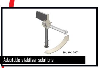
The stabilizer legs of the crane are to ensure stability - however they have to be easy to handle and must not take up too much space when not in use. Therefore you can choose between fixed stabilizer legs, manual swing-up stabilizer legs to 30/60° or manual swing-up stabilizer legs to 180° with gas spring. Stabilizer beams can be freely selected as hydraulically extensible or manually extensible, also in connection with the sophisticated EVS stability monitoring.
