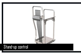
With stand-up control, the crane operator has an increased overview of the crane movements. Especially when loading and unloading the platform body with e.g. grab or pallet fork, the crane operator has the full view of both the platform body and the working area. The crane operator is protected by the HSL or HSL-E safety system which prevents the crane from hitting the operator on the stand-up platform.
