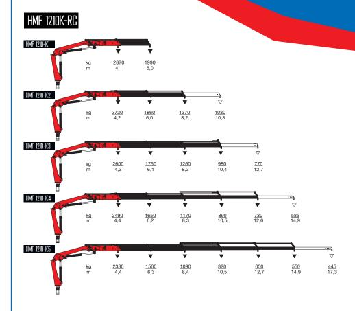
▼ Lifting capacity without manual extensions▽ Lifting capacity with manual extensions
