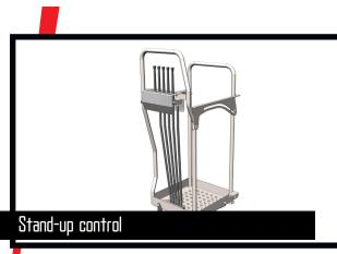
With stand-up control, the crane operator has an increased overview of the crane movements. Especially when loading and unloading the platform body with e.g. grab or pallet fork, the crane operator has the full view of both the platform body and the working area. The crane operator is protected by the HSL or HSL-E safety system which prevents the crane from hitting the operator on the stand-up platform.
