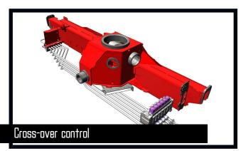
The lever sequence on manually operated cranes with ground control (JS) can be transferred via cross-over control rods to the opposite side of the crane. Thanks to cross over controls, you obtain that the control lever sequence is the same in both sides of the crane, i.e. the sequence is from the left: "Slew", "boom", "jib" and "extension". The rods are made of particularly sturdy steel pipes for precise and efficient control of the movements.
