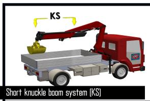
The short knuckle boom system (KS) is equipped with a shorter jib than a standard knuckle-boom system. Thanks to a short knuckle boom system, the crane fitted with a grab, can be stowed while extended in a platform body of 4 m without dismounting the grab. The lifting height close to the column is increased with more than 3 m and in this way offers the possibility of lifting tall items close to the column. The boom system is available with 1, 2 or 3 hydraulic extensions.
