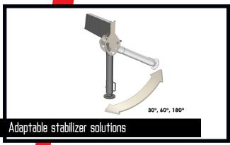
The stabilizer legs of the crane are to ensure stability - however they have to be easy to handle and must not take up too much space when not in use. Therefore you can choose between fixed stabilizer legs, manual swing-up stabilizer legs to 180° with gas spring or fully hydraulic swing-up stabilizer legs to 180°. Stabilizer beams can be freely selected as hydraulically extensible or manually extensible, also in connection with the sophisticated EVS stability monitoring.
