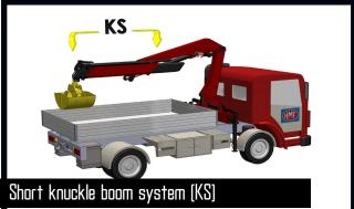
The short knuckle boom system (KS) is equipped with a shorter jib than a standard knuckle-boom system. Thanks to a short knuckle boom system, the crane fitted with a grab, can be stowed while extended in a platform body of 4 m without dismounting the grab. The lifting height close to the column is increased with more than 3 m and in this way offers the possibility of lifting tall items close to the column. The boom system is available with 1, 2 or 3 hydraulic extensions.
