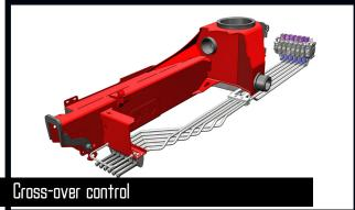
The lever sequence on manually operated cranes with ground control (JS) can be transferred via cross-over control rods to the opposite side of the crane. Thanks to cross-over controls, you obtain that the control lever sequence is the same in both sides of the crane, i.e. the sequence is from the left: "Slew", "boom", "jib" and "extension". The rods are made of particularly sturdy steel pipes for precise and efficient control of the movements.
