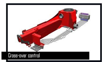
The lever sequence on manually operated cranes with ground control (JS) can be transferred via cross-over control rods to the opposite side of the crane. Thanks to cross-over controls, you obtain that the control lever sequence is the same in both sides of the crane, i.e. the sequence is from the left: "Slew", "boom", "jib" and "extension". The rods are made of particularly sturdy steel pipes for precise and efficient control of the movements.
