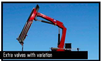
A well-known and usual hose routing to the end of the extensions means that 1 or 2 extra valves are fed in sturdy hose guides alongside the jib extension system. If further efficient protection of the hoses is required, 1 or 2 extra valves can be fed in internal hose reels and lie particularly well protected.
