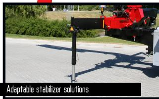
The stabilizer legs of the crane are to ensure stability - however they still have to be sturdy, easy to handle and must not take up too much space when not in use. Therefore you can choose between fixed stabilizer legs, manual swing-up stabilizer legs to 30/60° or manual swing-up stabilizer legs to 180° with gas spring. Stabilizer beams can be freely selected as hydraulically extensible or manually extensible, also in connection with the sophisticated EVS stability monitoring.
