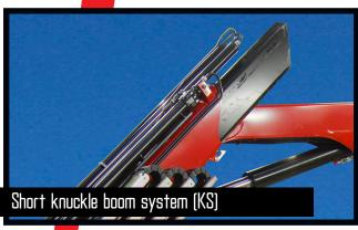
The short knuckle boom system (KS) is equipped with a shorter jib than a standard knuckle-boom system. Thanks to a short knuckle boom system, the crane fitted with a grab, can be stowed while extended in a platform body of 4 m without dismounting the grab. The lifting height close to the column is increased with more than 3 m and in this way offers the possibility of lifting tall items close to the column. The boom system is available with 1, 2 or 3 hydraulic extensions.
