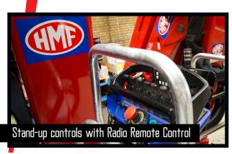
With stand-up controls and radio remote controls the crane operator has an increased overview of the crane movements. The remote control is placed in a bracket on the stand-up platform where it is fixed whilst operating the crane. The crane operator is protected by the HSL or HSL-E safety system which prevents the crane from hitting the operator on the stand-up platform.
