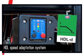
HDL-d is an electronic system which automatically adapts the crane speed to the working situation. You thus avoid big and sudden stress, which may damage the crane or influence the stability of the vehicle in an unfavourable way. The RCL 5300 is monitoring which movements that have to be adapted.
