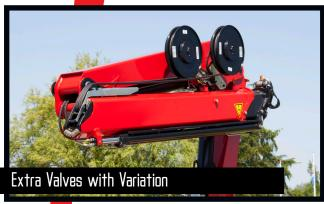
A well-known and usual hose routing to the end of the extensions means that 1 or 2 extra valves are fed in sturdy hose guides alongside the jib extension system. If further efficient protection of the hoses is required, 1 or 2 extra valves can be fed in internal hose reels and lie particularly well protected. In case of more than 6 hydraulic extensions or a reach of approx. 17 m, 1 or 2 extra valves will be fed in external, smooth-running and efficient hose reels.
