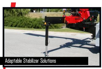
The stabilizer legs of the crane are to ensure stability - however they still have to be easy to handle and must not take up too much space when not in use. Therefore you can choose between fixed stabilizer legs, manual swing-up stabilizer legs to 180° with gas spring or fully hydraulic swing-up stabilizer legs to 180°. Stabilizer beams can be freely selected as hydraulically extensible or manually extensible, also in connection with the sophisticated EVS stability monitoring.
