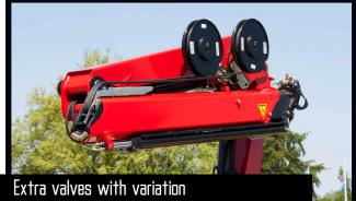
A well-known and usual hose routing to the end of the extensions means that 1 or 2 extra valves are fed in sturdy hose guides alongside the jib extension system. If further efficient protection of the hoses is required, 1 or 2 extra valves can be fed in internal hose reels and lie particularly well protected. In case of more than 6 hydraulic extensions or a reach of approx. 17 m, 1 or 2 extra valves will be fed in external, smooth-running and efficient hose reels.
