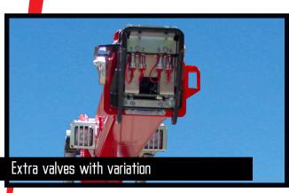
Extra valves (2 pcs.) are fed internally in the extension system in sturdy and efficient nylon drag chains in the jib extension system.
