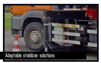
The stabilizer legs of the crane are to ensure stability - however they still have to be sturdy, easy to handle and must not take up too much space when not in use. Therefore you can choose between fixed stabilizer legs, manual swing-up stabilizer legs to 180° with gas spring or fully hydraulic swing-up stabilizer legs to 180°. Stabilizer beams can be freely selected as hydraulically extensible or manually extensible and also in connection with the sophisticated EVS stability monitoring system.
