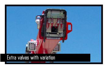
Extra valves (2 pcs.) are fed internally in the extension system in sturdy and efficient nylon drag chains in the jib extension system.
