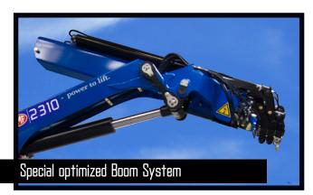
The HMF 2310-RCS is equipped with a specially developed boom system, which is particularly adapted to work with underground refuse containers (Molok deep collection containers). With 3 or 4 hydraulic extensions giving a reach of up to 11 m, the crane has a very large efficient working area. The compact geometric design and optimized installation height only take up minimum space and the crane can therefore easily be stowed over a compactor.
