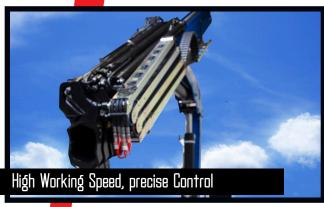
With the Danfoss PVG 32 control valve the HMF 2310S-RCS obtains very high working speeds without compromising neither safety nor precision. A hydraulic pump flow of up to 120 I/min and a variable flow pump, which at the same time is very energy-efficient, means all in all lower costs, because a short working cycle results in more collections per day.
