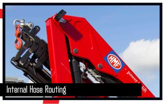
Internal hose routing both through the column and stabilizer beams gives the crane an elegant design which also provides maximum protection for the hoses from wear, sunlight and other mechanical stress.
