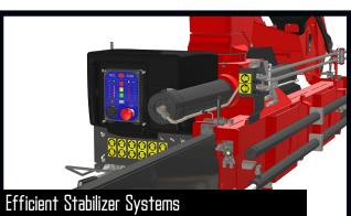
The double cross beam offers the best conditions for a stable and flexible stabilizer concept with a large stabilizer spread with type "S" single beams or type "D" double beams. Also available as an option with hydraulically extensible stabilizer beams operated from a separate valve block placed on the cross beam of the crane.
