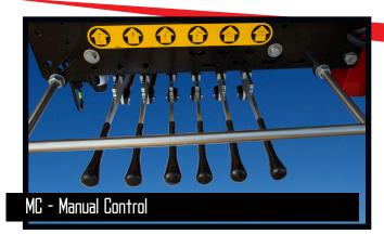
The crane is equipped with a manually operated control valve providing precise and simple control of the crane functions. The RCL 5300 TCL Safety System will only limit the load moment increasing movements if the crane reaches 100% capacity - all other functions remain fully operational.
