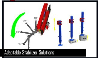
The crane's stabilizer legs are robust, easy to handle and require minimum space. You can choose between fixed stabilizer legs or manual swing-up stabilizer legs ( $45^\circ$ ,  $90^\circ$ ,  $135^\circ$ ,  $180^\circ$ ) with or without gas spring. The stabilizer cylinder is adjustable by +/- 200 mm in height, with full stroke.
