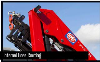
Internal hose routing both through the column and stabilizer beams gives the crane an elegant design which also provides maximum protection for the hoses from wear, sunlight and other mechanical stress.
