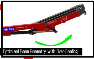
The boom system is equipped with single Power Plus link arm system on the jib, allowing a maximum load moment with stretched boom system. It is additionally fitted with a "genuine" HMF over-bending of 15° which means that the crane is capable of lifting the maximum capacity in the maximum over-bending position.
