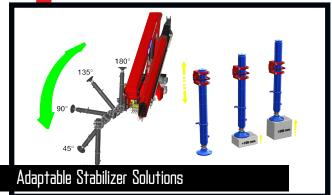
The crane's stabilizer legs are robust, easy to handle and require minimum space. You can choose between fixed stabilizer legs or manual swing-up stabilizer legs ( $45^\circ$ ,  $90^\circ$ ,  $135^\circ$ ,  $180^\circ$ ) with or without gas spring. The stabilizer cylinder is adjustable by +/- 200 mm in height, with full stroke.
